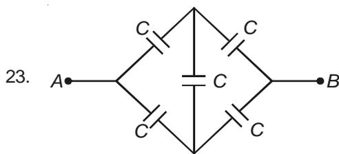
Capacity of the arrangement across  $AB$  as shown in figure
